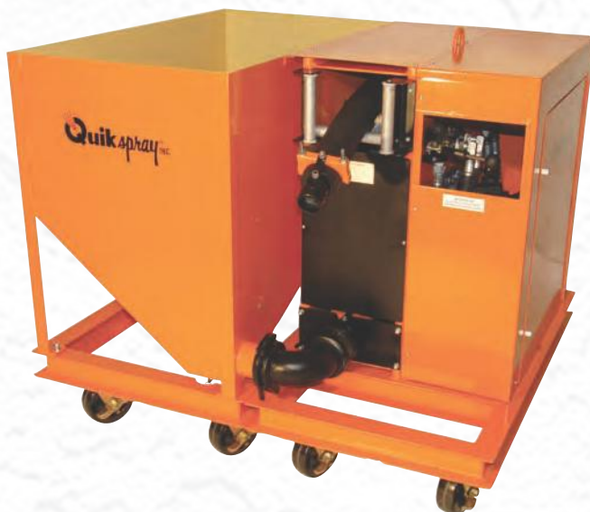
2" I.D. Hydraulic or Electric with removable hopper
