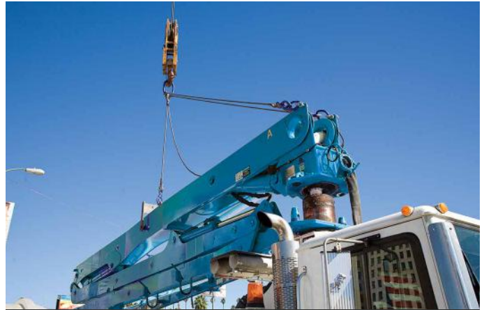
STEP 2 – Detach boom and lift
