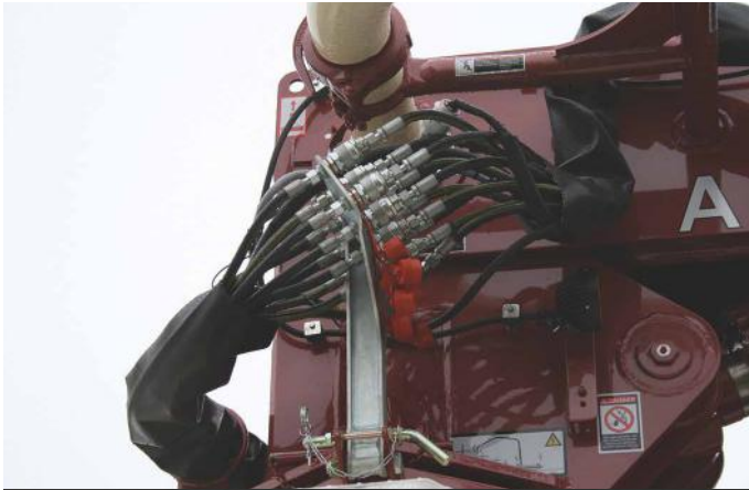
STEP 1 – Hydraulic Connection
