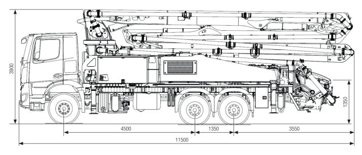
Note: Standard version. Dimensions and weights depend on truck, pump model and equipment. Dimensions in mm for MB-Arocs 2640. Illustrations show special equipment.
